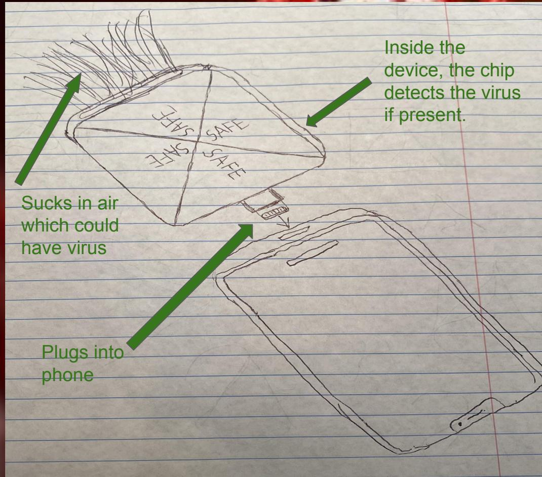
The VIRUSafe will be used for coronavirus detection, but it can be used for future virus outbreaks. The device will use the following components for detecting the virus:
