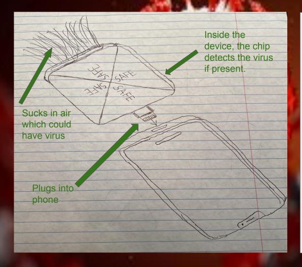
The VIRUSafe will be used for coronavirus detection, but it can be used for future virus outbreaks. The device will use the following components for detecting the virus:
